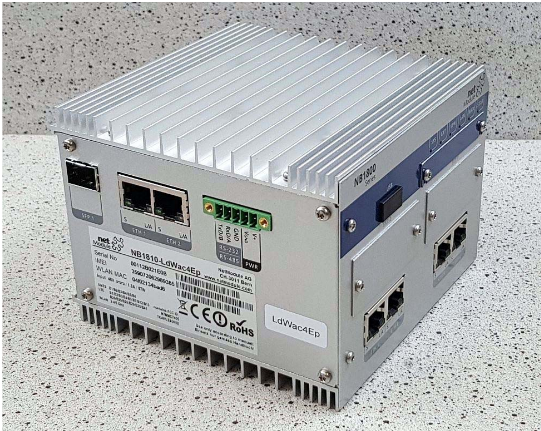
Interfaces of NB1810 (power, serial and LAN)
