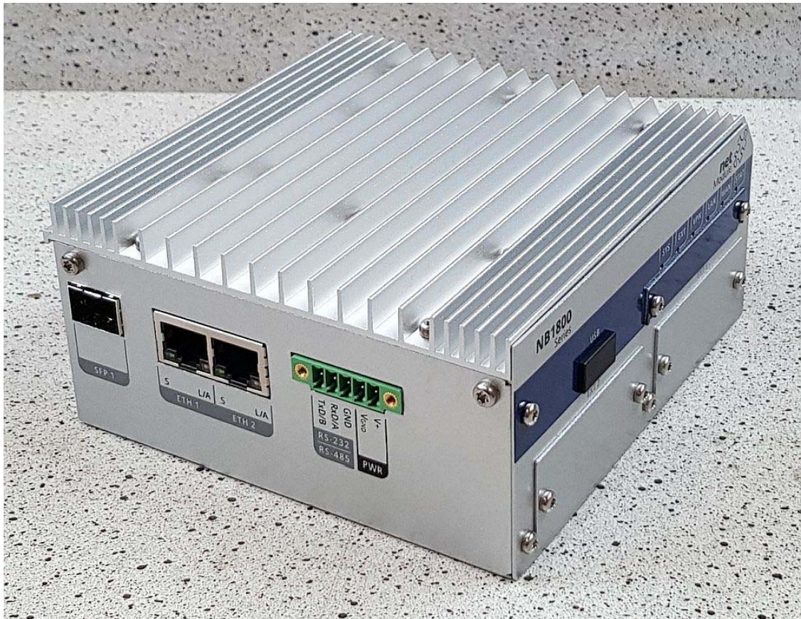
Interfaces of NB1800 (power, serial and LAN)
