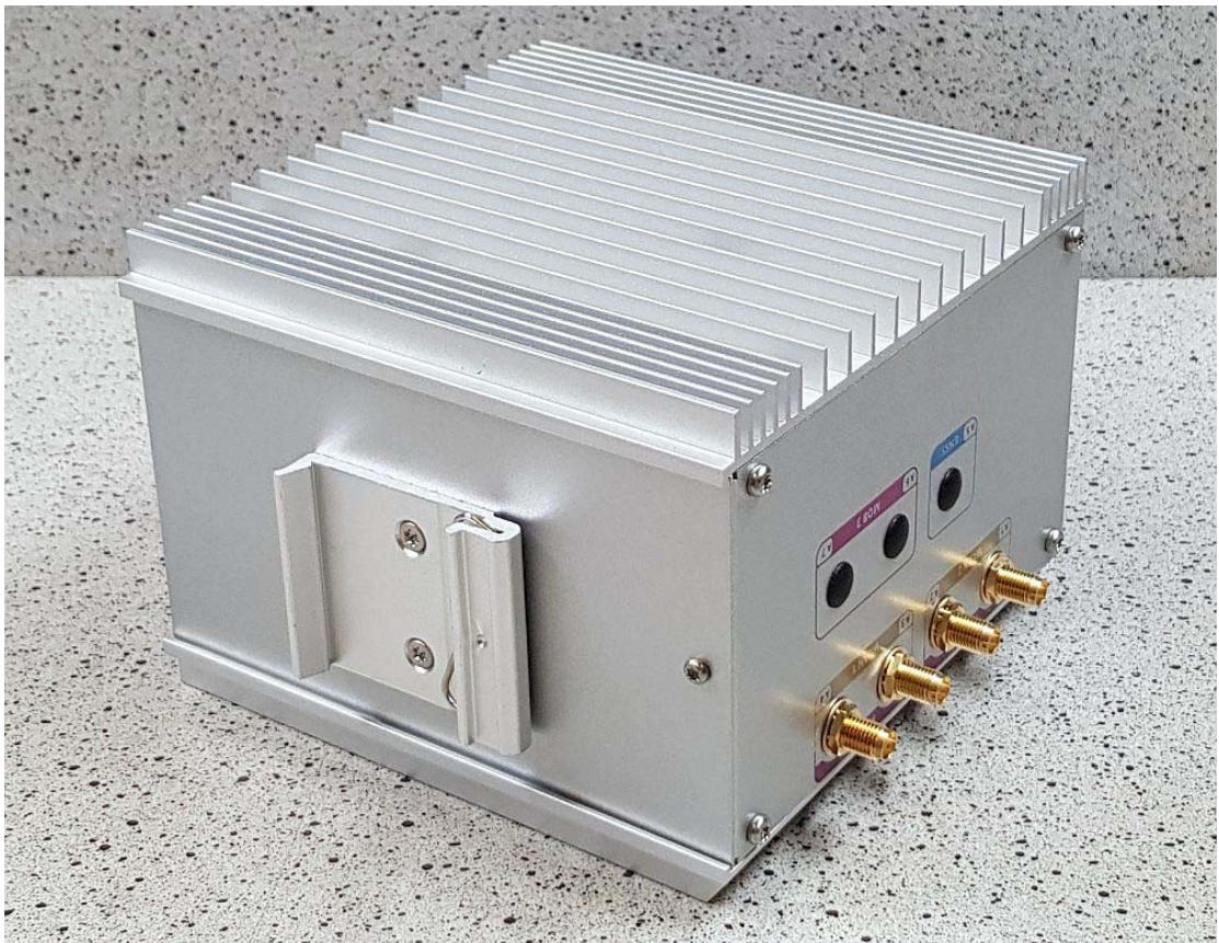
Rear view of NB1810 (DIN rail mounting), antenna connectors on the right
